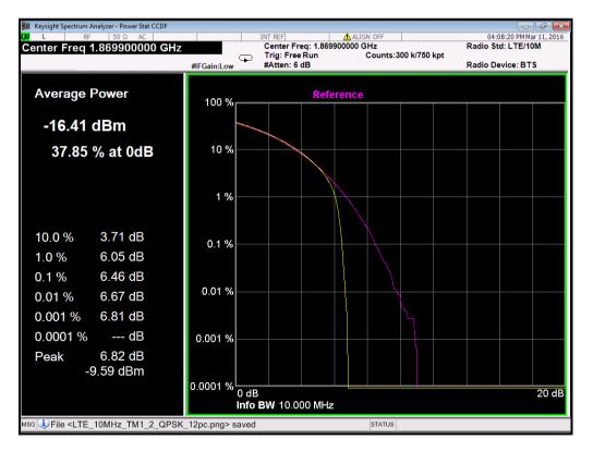
Figure 2: CCDF for 10 MHz LTE, TM1.2 with 12% EVM.
